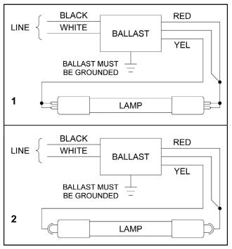
NOTE: For 4-Pin Single Ended Lamps, See Wiring Diagram Below.
