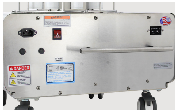
Location of Danger Labels (70-0036, 70-0037, and 70-0011) on Back of Unit
